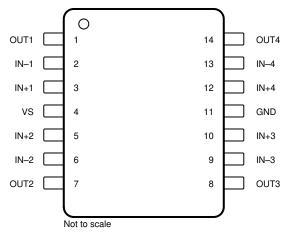
Figure 6-5. INA4180: PW Package 14-Pin TSSOP Top View
