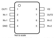
Figure 6-3. INA2180: DGK Package 8-Pin VSSOP Top View
