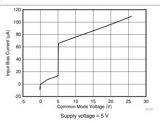
Figure 7-20. Input Bias Current vs. Common-Mode Voltage
