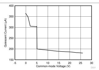
Figure 7-26. Quiescent Current vs. Common-Mode Voltage (INA180)
