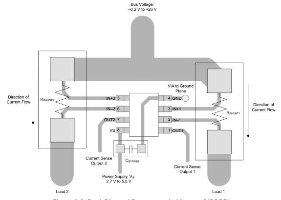
Figure 9-8. Dual-Channel Recommended Layout (VSSOP)
