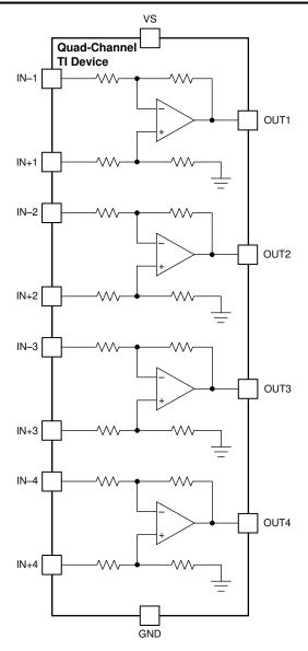
Figure 8-3. INA4180 Functional Block Diagram
