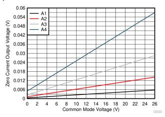
Figure 8-5. Zero-Current Output Voltage vs Common-Mode Voltage
