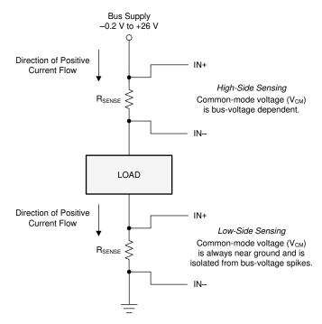
Figure 8-4. High-Side and Low-Side Sensing Connections
