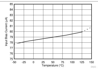
Figure 7-22. Input Bias Current vs. Temperature
