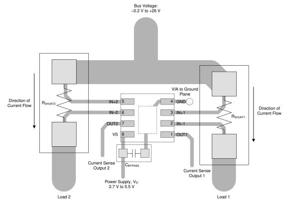
Figure 9-9. Dual-Channel Recommended Layout (WSON)
