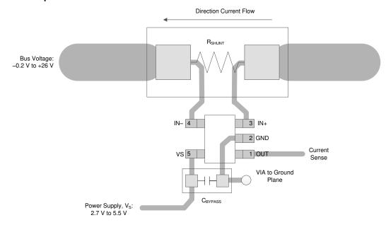
Figure 9-7. Single-Channel Recommended Layout (Pinout A)
