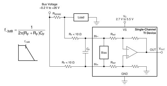
Figure 9-2. Filter at Input Pins
