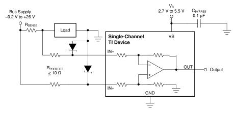
Figure 9-5. Transient Protection Using Dual Zener Diodes
