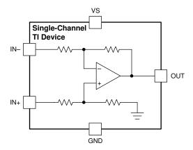
Figure 8-1. INA180 Functional Block Diagram
