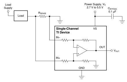
Figure 9-3. Low-Side Sensing
