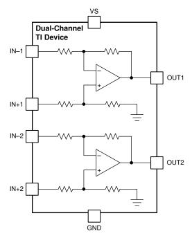
Figure 8-2. INA2180 Functional Block Diagram
