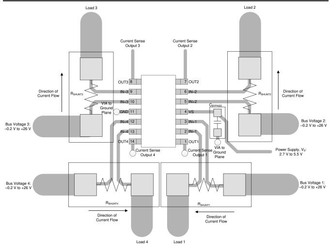
Figure 9-10. Quad-Channel Recommended Layout
